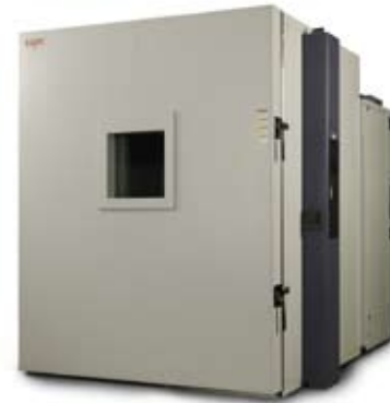
Solid walk-in chambers like this one are commonly selected for full-size solar panel testing.
