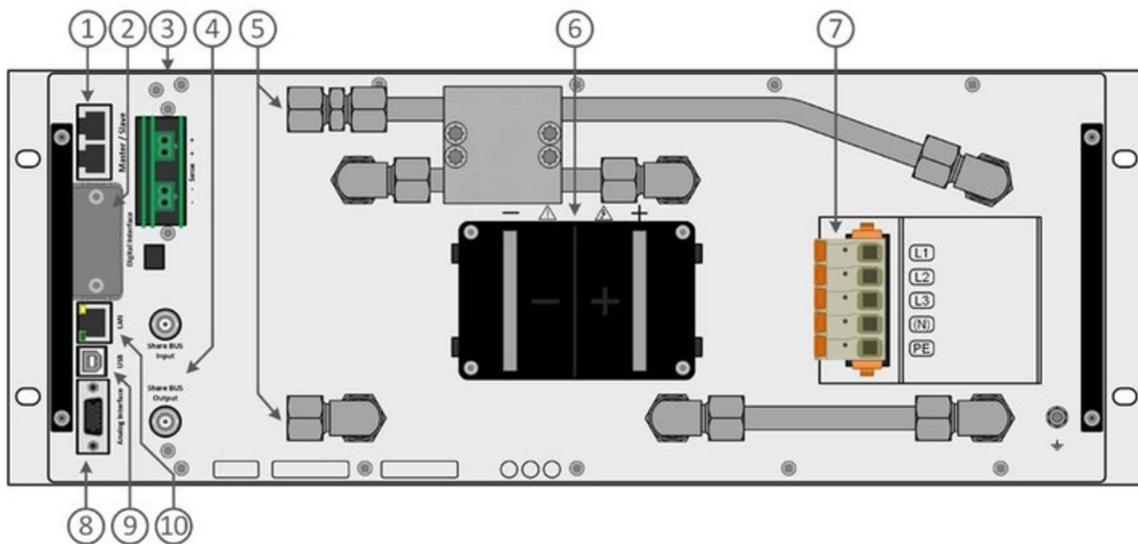
1. Master-Slave-Bus connectors to set up a system for parallel connection
