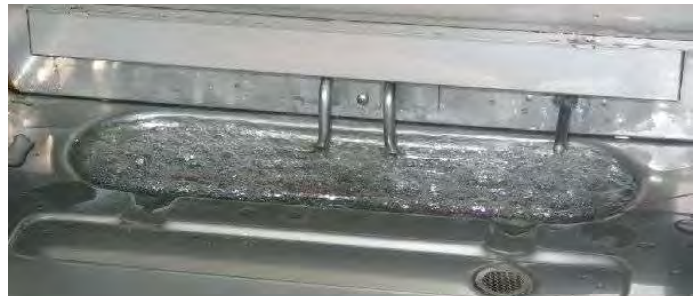
A humidity bath heats water right in the chamber for faster response, and is easier to maintain than traditional steam generators.
