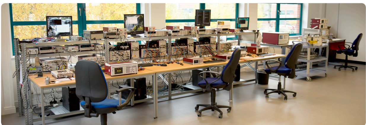
Section of the N4L UK Calibration laboratory with 7 of total 12 ACCIV calibration systems and Fluke 6105A Electrical Power Standard
