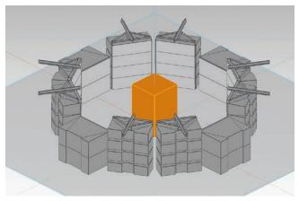
Minisatellite testing: loudspeakers circularly positioned around the specimen to create a sound pressure field
