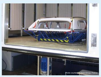
Combined climatic and vibration testing of car sunroofs
