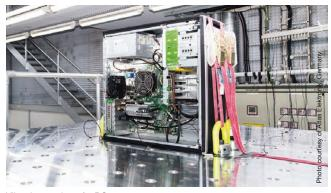
Vibration testing of a PC
