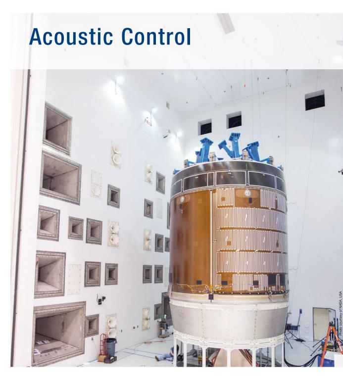
m+p international is considered the market leader for reverberant chamber excitation. Our m+p VibControl performs acoustic testing in reverberant chambers and direct field environments as well as progressive wave tube testing. It is a fully automatic digital control system, providing fast, accurate and repeatable control of highlevel noise to a reference octave band spectrum and the overall sound pressure level (OASPL). The control guarantees a high level of product safety.
