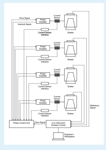
Schematic functioning diagram
