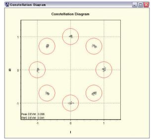
BlueSuite Pro3 displays the IQ constellation pattern for all payload symbols, or any user defined 50  $\mu$ s block. Limit circles are preset to the core specification requirement for  $\pi/4DQPSK$  or 8DPSK modulation standards.
