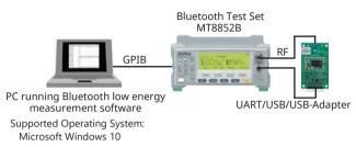
Use of the Bluetooth low energy software provides the ideal environment for detailed graphical analysis of Bluetooth low energy packets. Devices with an HCI interface can be tested automatically by configuring and running an automated test script from the PC.
